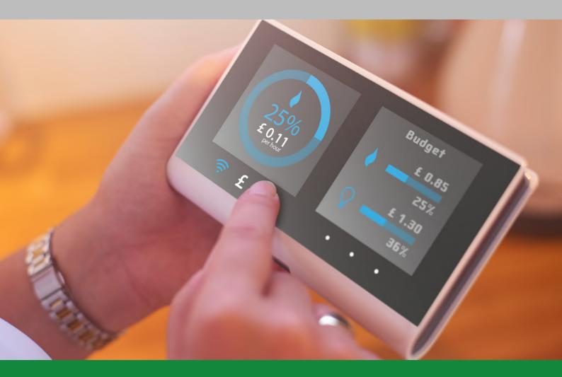
Smart meters measure how much gas and electricity you're using via a remote connection to your energy supplier. They come with an in-home display which receives data from the meter and lets you see your energy usage and costs in real-time, helping you to manage energy consumption and spend more efficiently.
